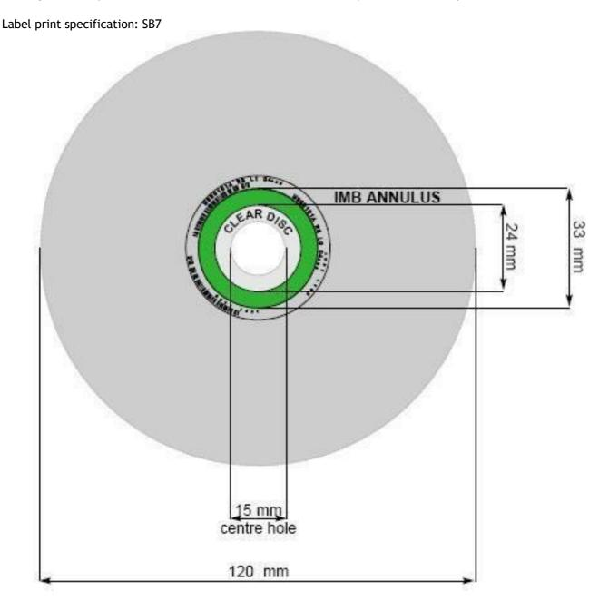
Inner Diameter: 34mm Outer Diameter: 116mm
